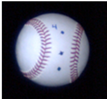
Figure 4. Image of tracking dots on baseball that were used to measure spin.
