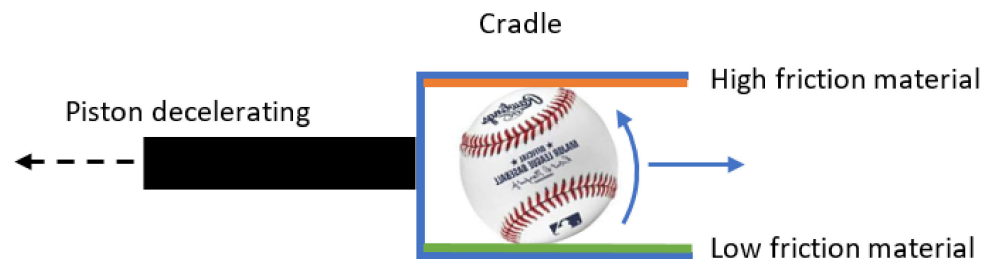
Figure 3. Schematic of the cradle attached to the pneumatic piston, showing spin imparted to the baseball as the piston decelerates.
