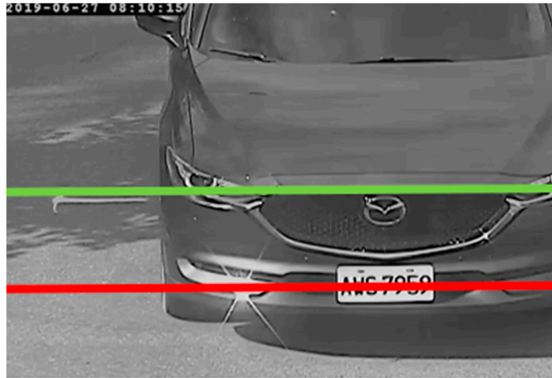
Figure 11. Virtual judgment line setting for license plate frames. Two virtual judgment lines (i.e., green and red lines) are used for license plate frames.
