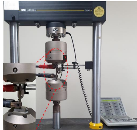
Figure 3. Test set-up for Fe-SMA activation.
