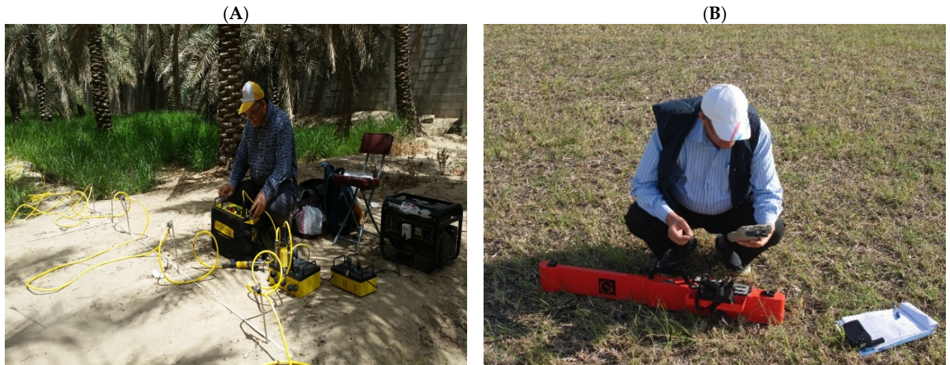
Figure 3. Geophysical data acquisition using the SuperSting R8/IP 8 resistivity (A) and the EM38-MK2 system electrical conductivities (B) at the study area.
