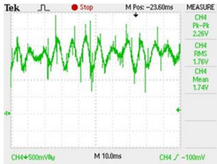
Figure 18. Torque ripple, normal operation, 2500 rpm, 3.5 Nm.
