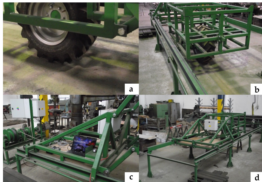
Figure 6. The process of measuring the rolling resistances of selected tires on the concrete surface of the laboratory. (a) View of the tested tire and concrete surface; (b) view of the main frame with the wheel; (c) location of the measuring apparatus on the guide frame; (d) general view of the experimental equipment.
