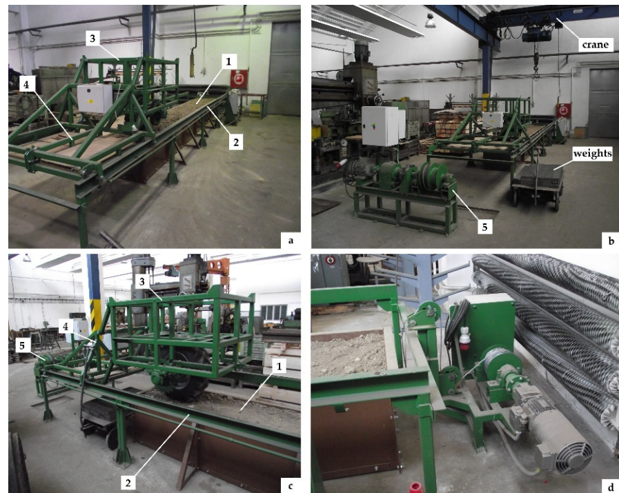
Figure 2. Soil test channel without wheel drive installation. (a) Workplace layout, (b) general view of the equipment with weights and handling crane, (c) detailed view of the main frame with the tested tire, (d) auxiliary return winch. 1. Ground channel; 2. Side guide; 3. Main frame with wheel; 4. Guide frame; 5. Braking and winding device.
