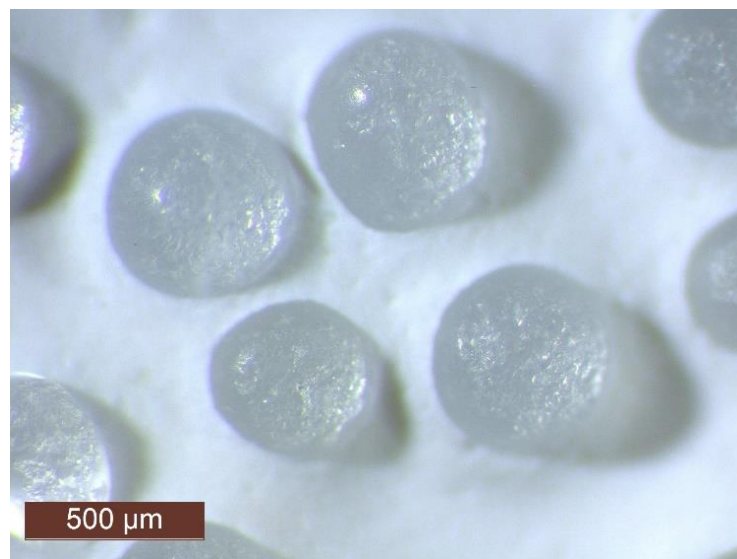
Figure 7. Exemplary severely damaged GB ( high index , sample HI) after exposure to 6720 drum rotations. Microscope image (magnification 32×).
