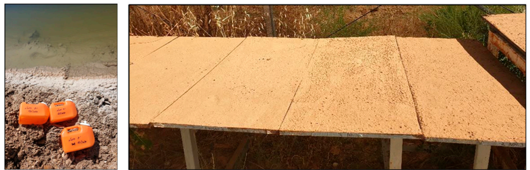
Figure 1. Samples of Dead Sea salt solutions collected in 3 L containers (left side) and trays of Ze'elim soil treated with different brines (surface area of 0.5 m \times 1.0 m and height of 0.02 m).
