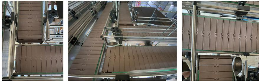
**Figure 27.** Perpendicular position between two conveyors.
