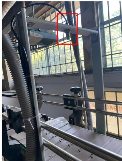
**Figure 28.** The installation position of proximity sensors on the sub-conveyors.
