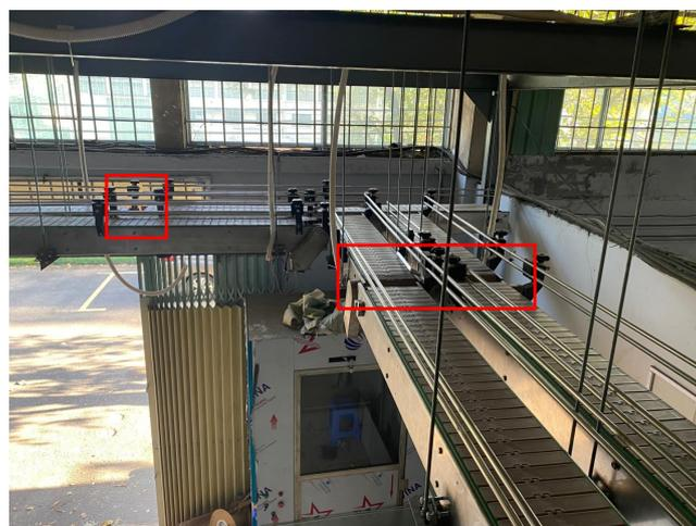
Figure 26. Transition position between two conveyors.
