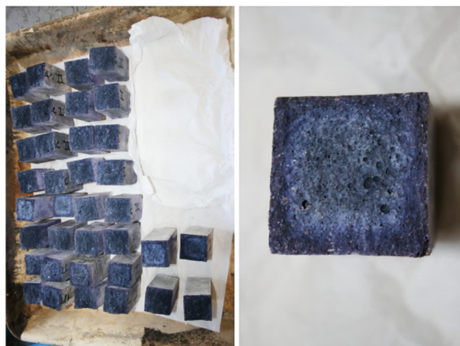
Figure 15. Sulphate penetration depth in tested mortars, using \text{BaCl}_2 + \text{KMnO}_4 solutions and after 6 months of immersion in a sodium sulphate solution.
