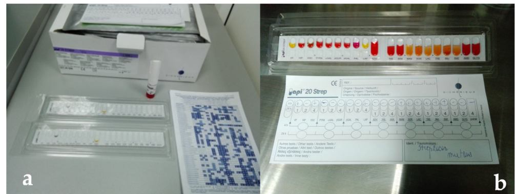
Figure 2. (a,b) API kit (Bio-Merieux, Craponne, France) for the identification of bacterial cultures.
