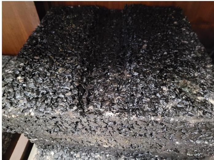
**Figure 8.** Photograph of a wheel track test sample made with the 1.5% GGBFS asphalt mixture.
