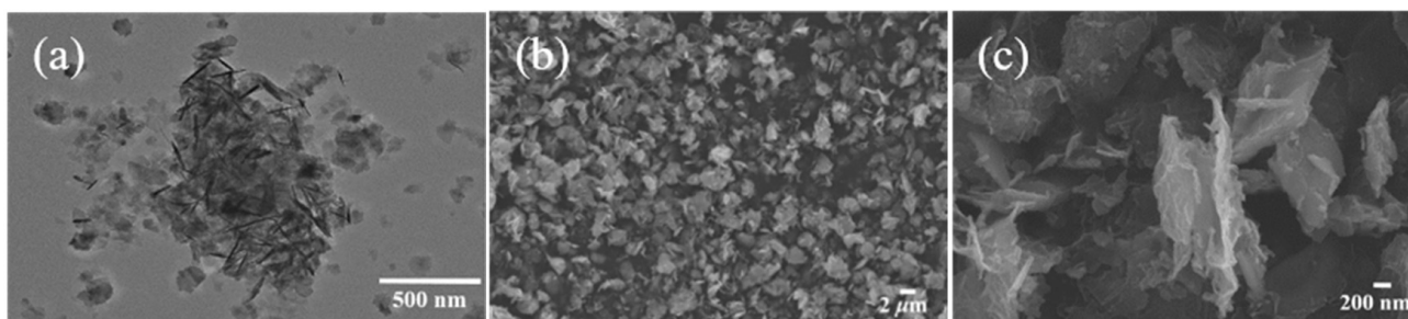
Figure 8. (a) TEM; (b) low-magnification and (c) high-magnification SEM images of the NiCo 2 S 4 /rGO composites.
