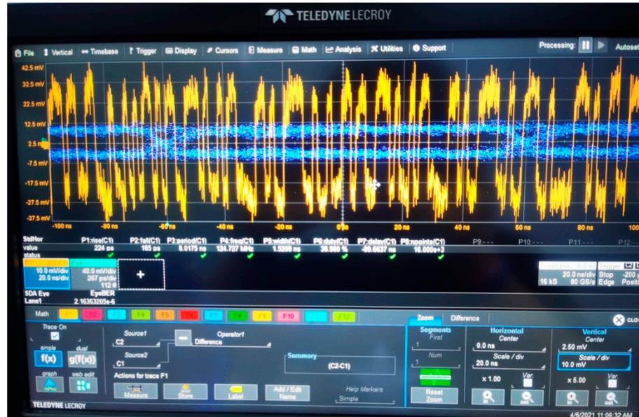
Figure 7. The eye diagram of experimental site at 8G communication frequency.
