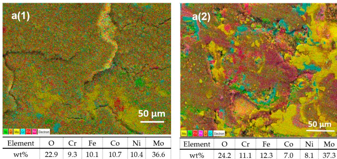
**Figure 14.** EDX mapping results (a) of the layer formed on the (a1) HVOF-HEA\_Mo<sub>27</sub> and (a2) HVOF-HEA\_Mo<sub>20</sub> as-sprayed coatings after 12,000 wear cycles under dry test condition.
