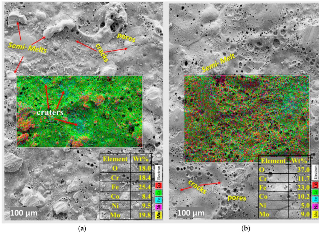
**Figure 3.** Top surface morphologies, elemental concentration and surface maps of the as-sprayed (a) ESD-HEA\_Mo<sub>27</sub>, (b) ESD-HEA\_Mo<sub>20</sub> coatings.
