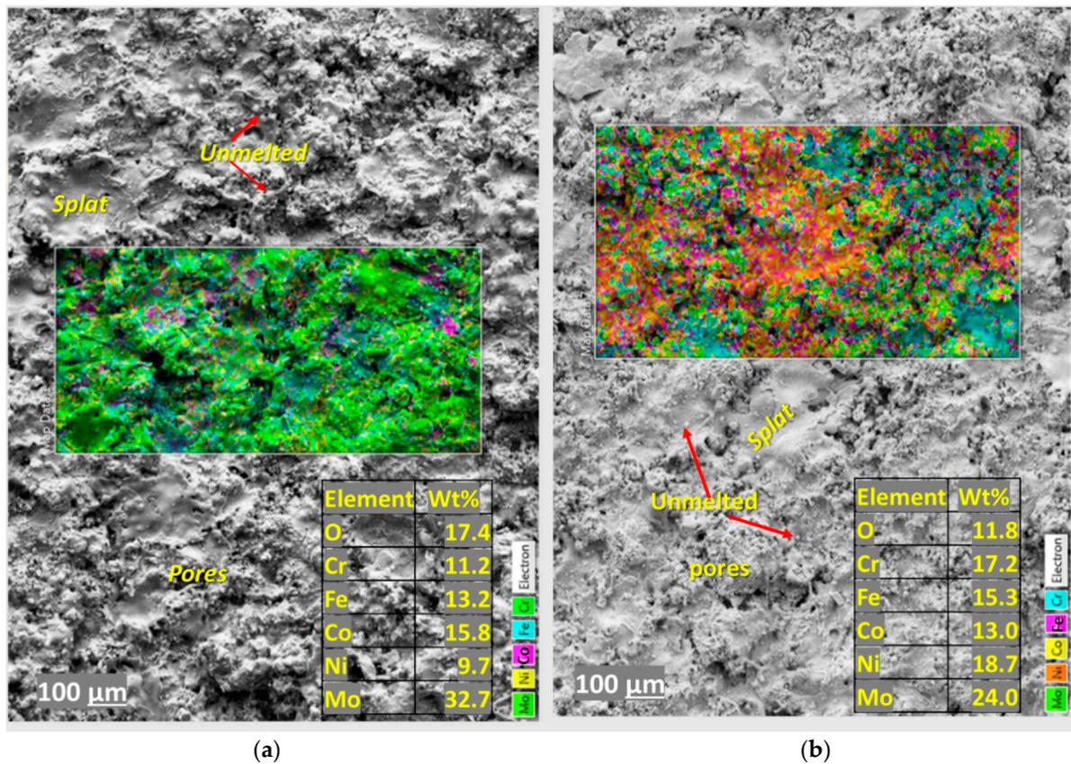
**Figure 1.** Top surface morphologies, elemental concentration and surface maps of the as-sprayed (a) HVOF-HEA\_Mo<sub>27</sub>, and (b) HVOF-HEA\_Mo<sub>20</sub> coatings.
