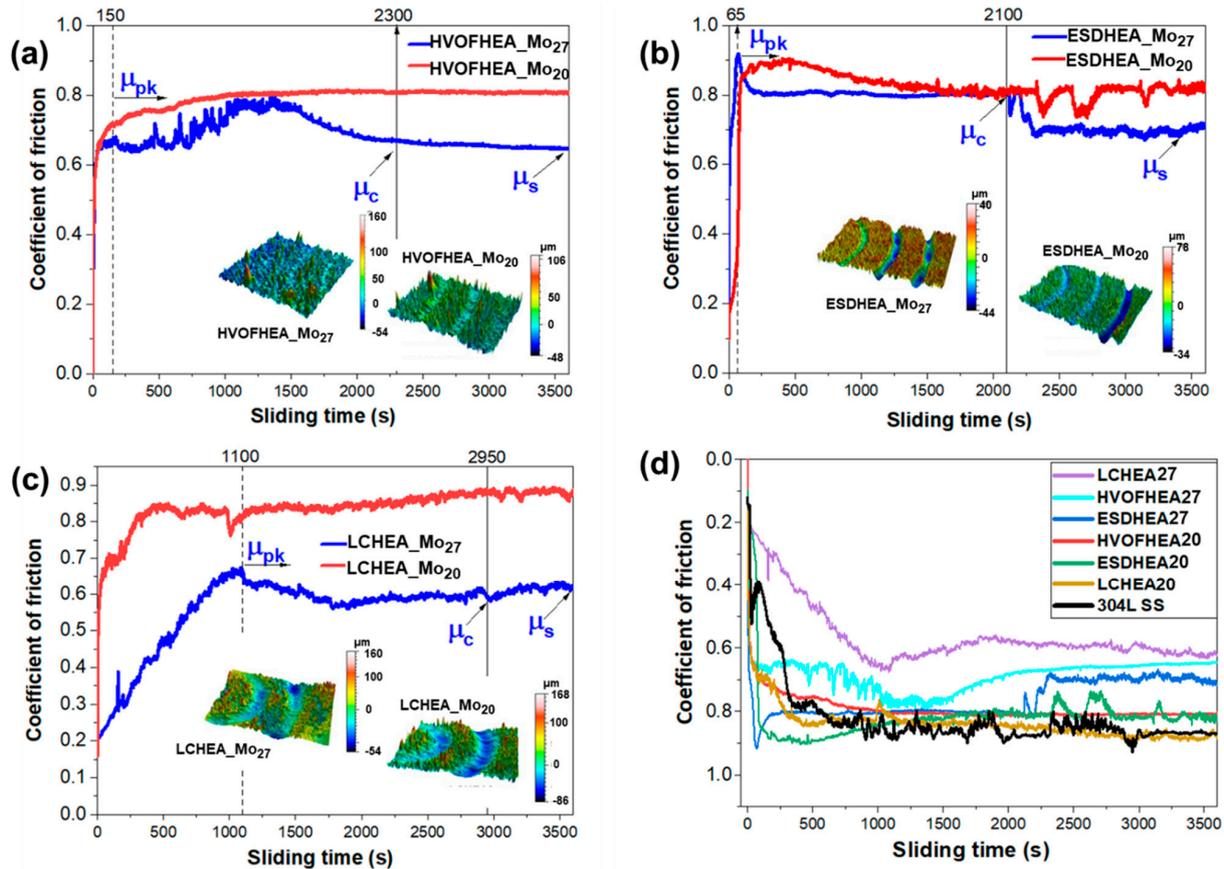
**Figure 9.** Evolution of coefficient of friction (CoF) versus sliding time after 12,000 wear cycles under dry test condition for the as-sprayed (a) HVOF, (b) ESD, (c) LC -HEA coatings and (d) 304L SS and HEACs with the different deposition techniques.
