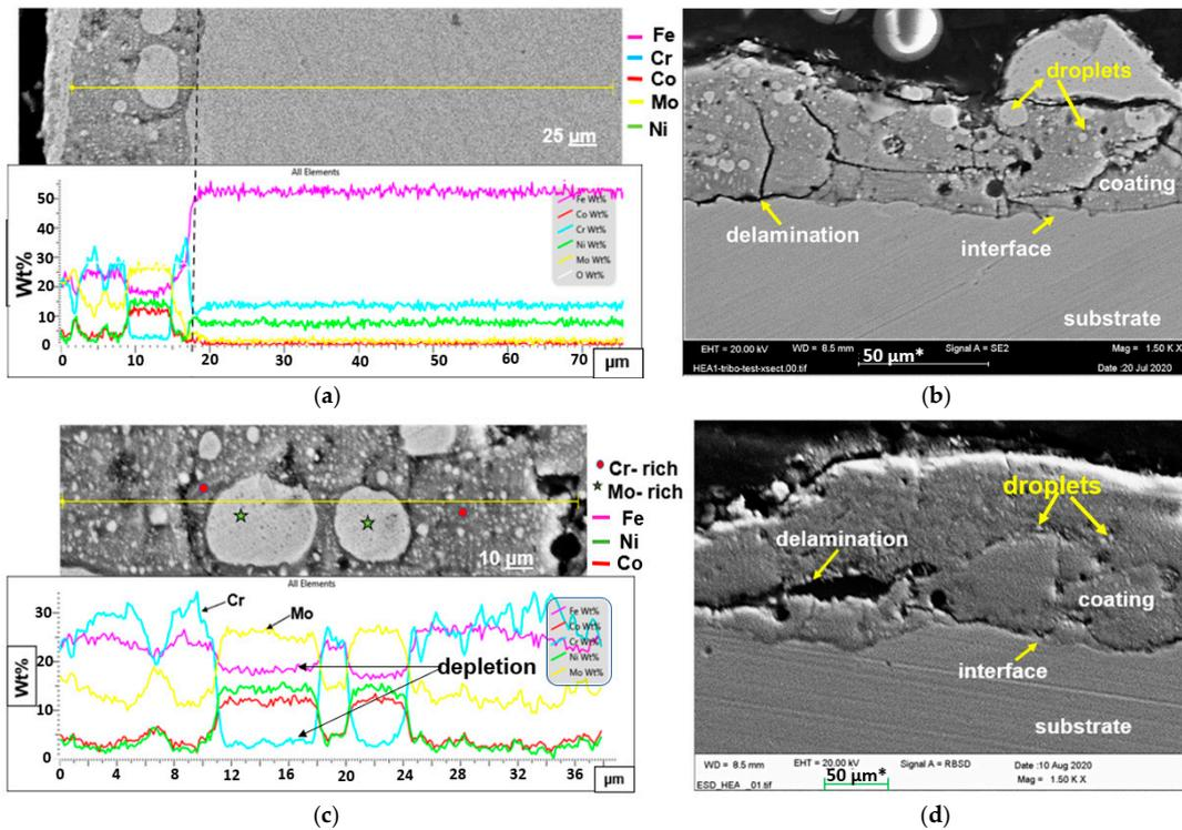
**Figure 4.** SEM and BSE micrographs of the cross-section and EDX line scans, revealing of the as-sprayed (a,b) ESD-HEA\_Mo<sub>27</sub> and (c,d) ESD-HEA\_Mo<sub>20</sub> coatings.
