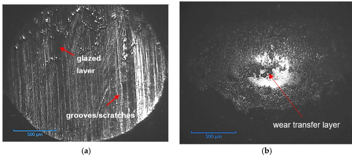
**Figure 11.** Optical micrographs of worn scars morphology of WC ball sliding against (a) HVOF-HEA\_Mo<sub>20</sub> and (b) LC-HEA\_Mo<sub>20</sub> coatings after 12,000 wear cycles under dry test condition.
