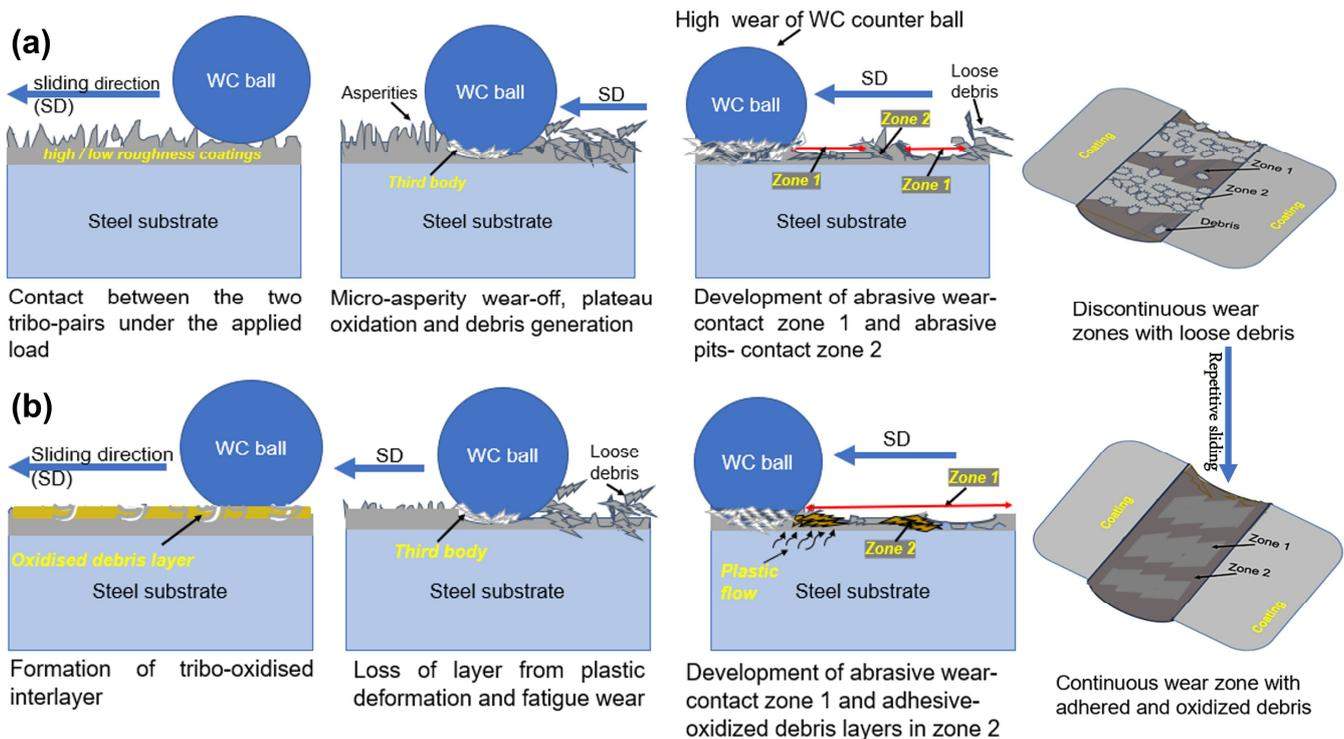
**Figure 15.** A schematic of the wear evolution proposed for the produced HEACs: (a) abrasive wear mode with plastic deformation and debris generation at the onset of sliding and (b) third body influence with subsequent decrease in the wear. Wear transition from mode (a) to (b) due to oxidation and repetitive sliding.
