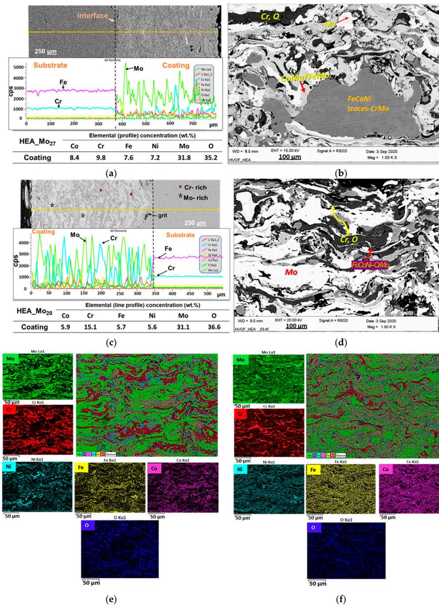
**Figure 2.** SEM (a,c) and BSE micrographs (b,d) of the cross-sections of the as-sprayed HVOF-HEA\_Mo<sub>27</sub> (a,b,e) and HVOF-HEA\_Mo<sub>20</sub> coatings (c,d,f) and the corresponding EDX line scans (a,c) and maps (e,f).
