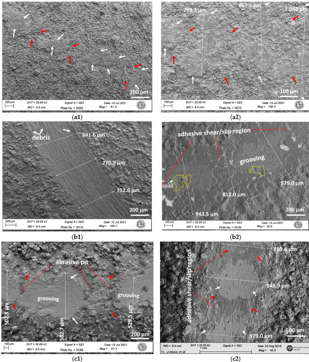
**Figure 12.** SEM micrographs of morphology of the wear tracks of the (a1) HVOF-HEA\_Mo<sub>27</sub>, (b1) ESD-HEA\_Mo<sub>27</sub>, (c1) LC-HEA\_Mo<sub>27</sub> and (a2) HVOF-HEA\_Mo<sub>20</sub>, (b2) ESD-HEA\_Mo<sub>20</sub>, (c2) LC-HEA\_Mo<sub>20</sub>—CoCrFeNiMo coatings with the different coating techniques after 12,000 wear cycles under dry test condition.
