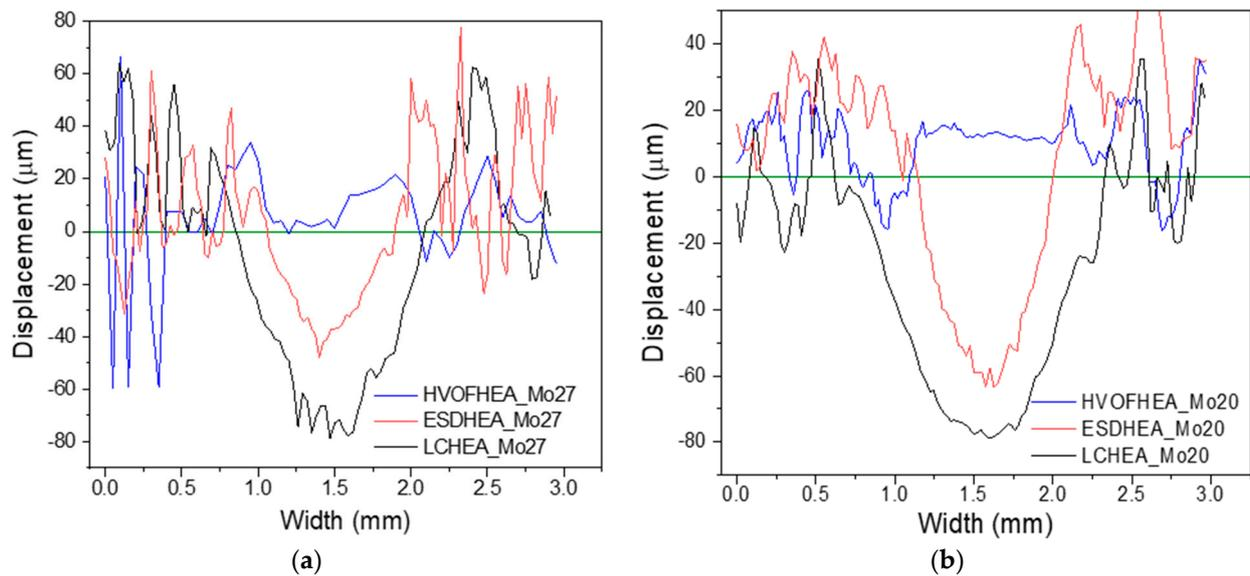
**Figure 10.** The topography profiles of the HEA coatings with the different deposition techniques after 12,000 wear cycles under dry test condition (a) HEA\_Mo<sub>27</sub> and (b) HEA\_Mo<sub>20</sub>.
