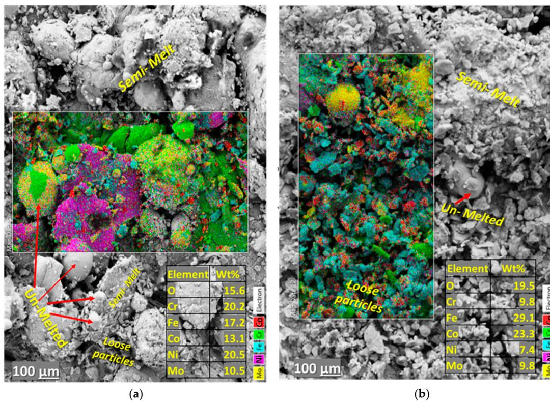
**Figure 5.** Top surface morphologies, elemental concentration and combined EDX surface map of the as-sprayed (a) LC-HEA\_Mo<sub>27</sub> and (b) LC-HEA\_Mo<sub>20</sub> coatings.
