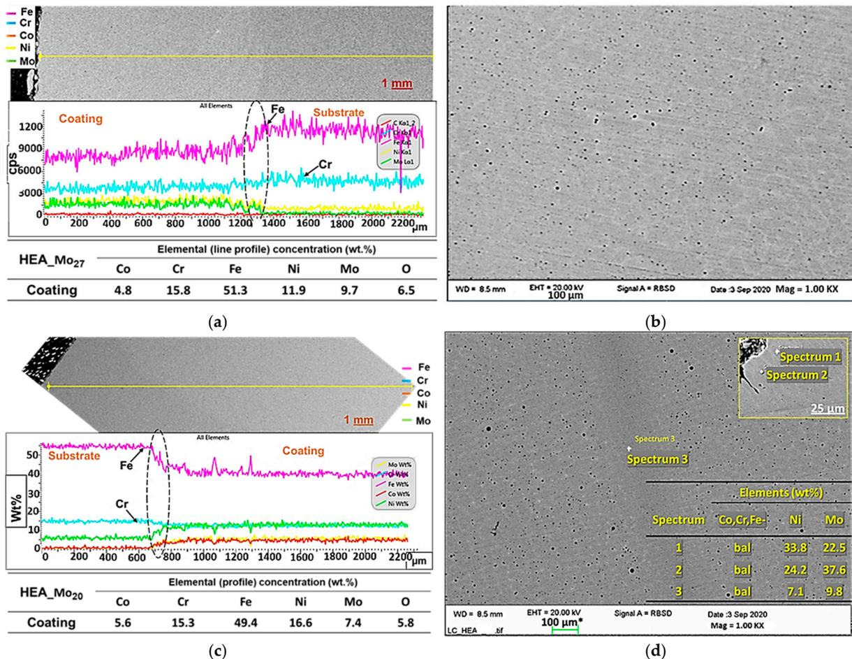
**Figure 6.** SEM and BSE micrographs of the cross-sections, and EDX line scans, point and area analysis of the as-sprayed (a,b) LC-HEA\_Mo<sub>27</sub> and (c,d) LC-HEA\_Mo<sub>20</sub> coatings.
