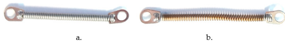
Figure 8. Ni-Ti spring after testing phase with I_1 current (a) and after testing phase I_2 current (b).
