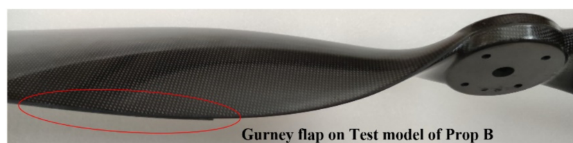
Figure 25. The detail of the Gurney flap on the test model.
