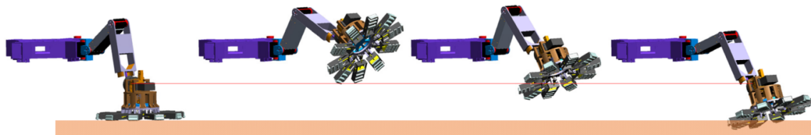
Figure 10. The motion process of the anchoring mechanism when stepping.
