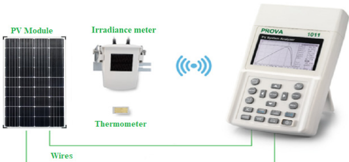
Figure 2. Set-up for extracting IV curves by Prova 1011 solar system analyzer.
