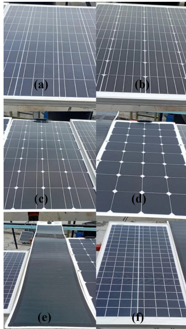
Figure 1. (a) Polycrystalline panel, (b) monocrystalline panel, (c) flexible mono-panel, (d) thin-film amorphous panel, (e) CIGS solar panel, and (f) flexible back-contact mono-panel.
