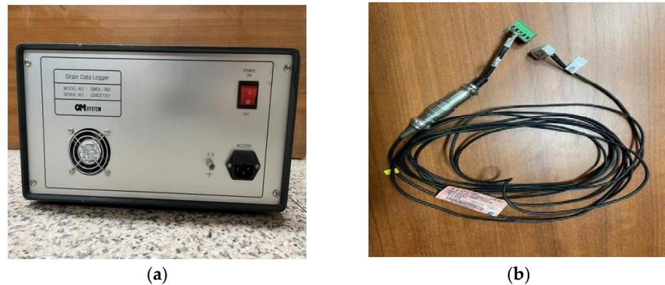
Figure 3. Acceleration capture instrument in this study: (a) Data logger; (b) Accelerometer.
