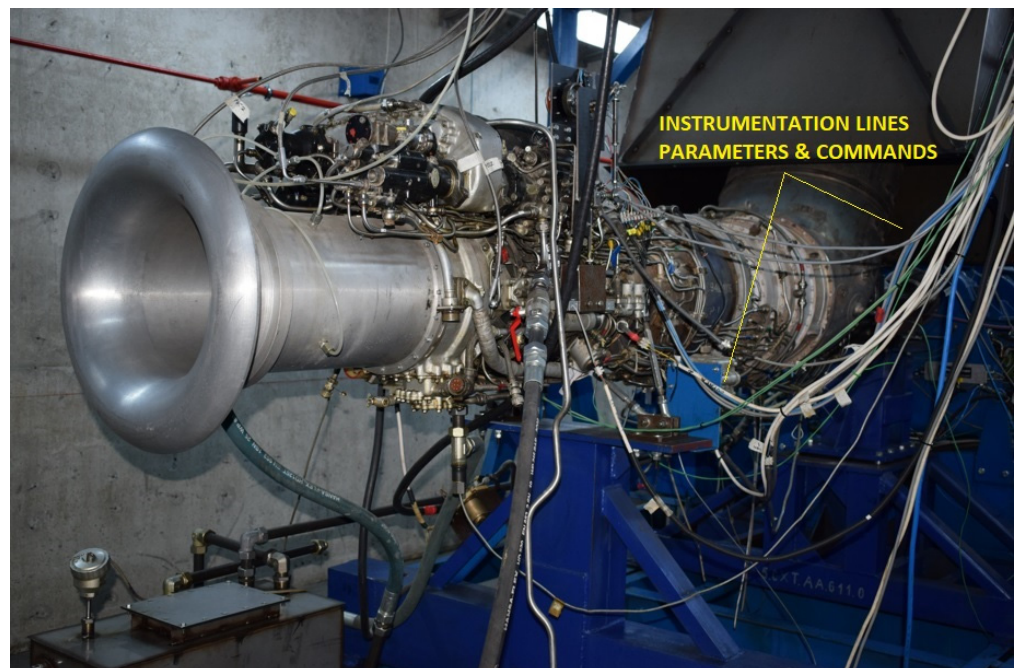
Figure 4. TV2-117A engine instrumentation lines.
