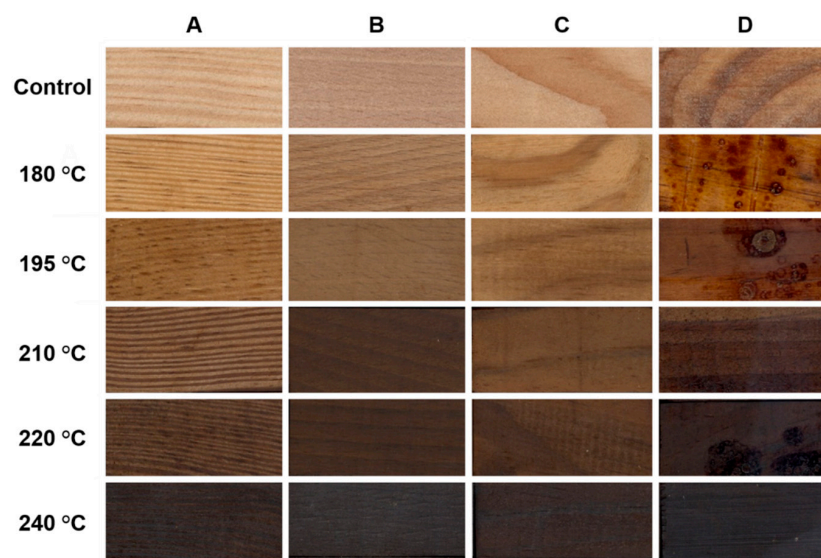
Figure 2. Thermally modified samples: Scots pine (A), beech (B), stone pine sapwood (C), stone pine heartwood (D).
