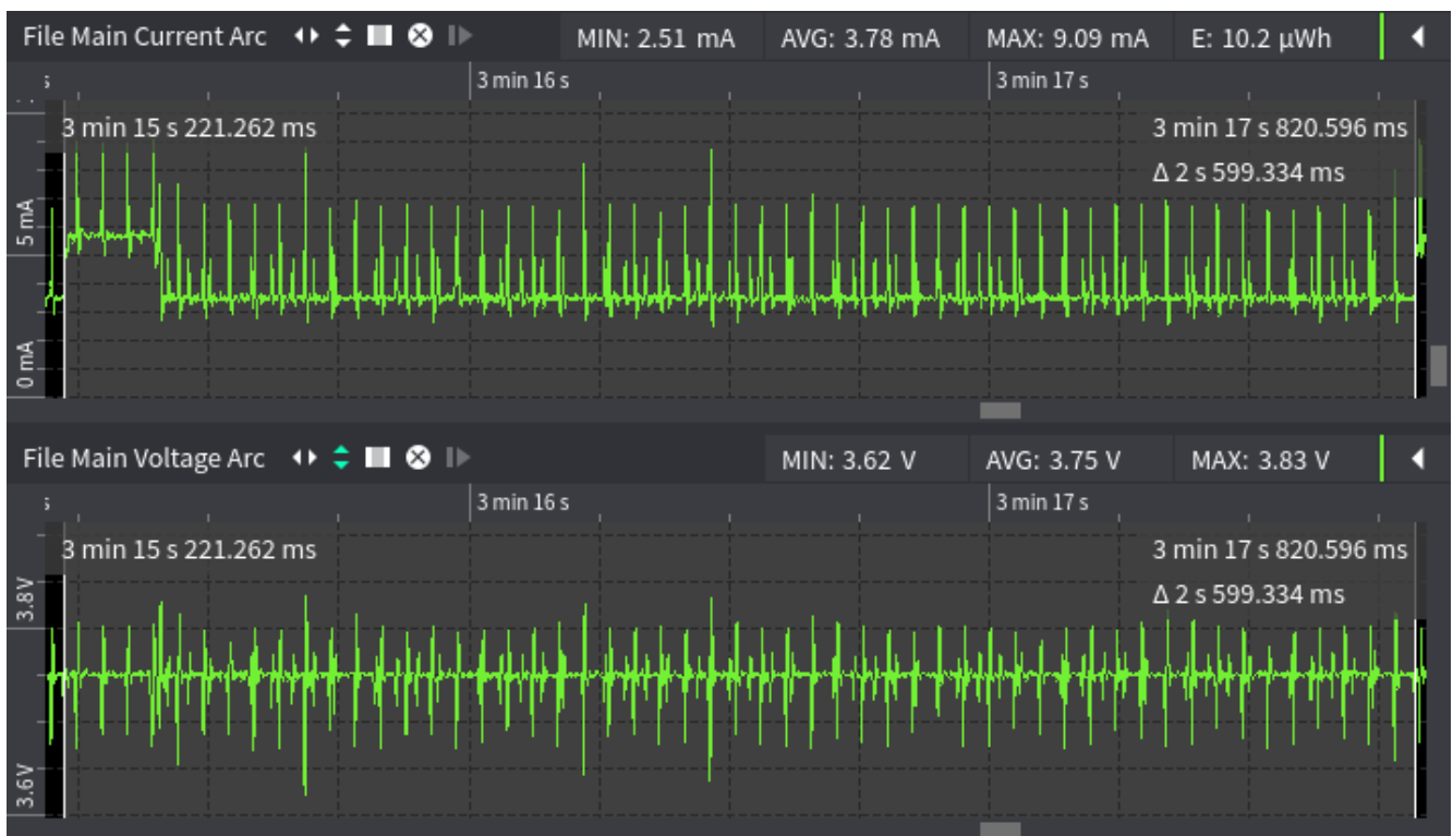
Figure 9. Current and voltage captures over one inference period by Qoitech Oti software for int16 model with 48 filters per convolution and CMSIS-NN optimizations
