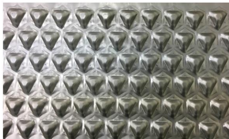
Figure 13. Formed truss score panel using the progressive press-forming method.
