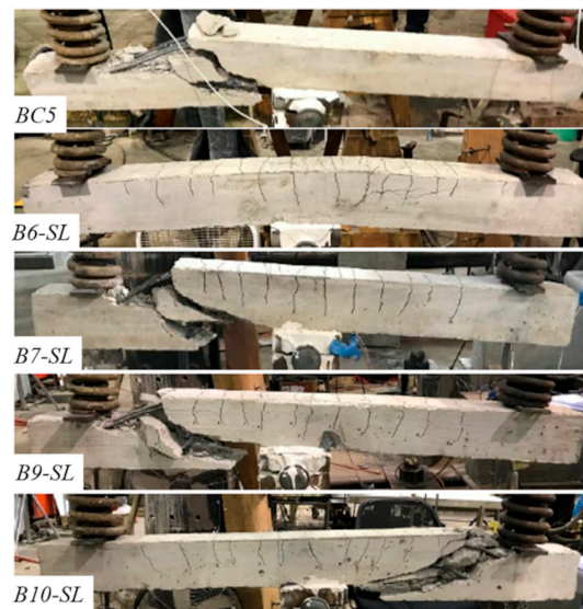
Figure 12. Beam series II failures.
