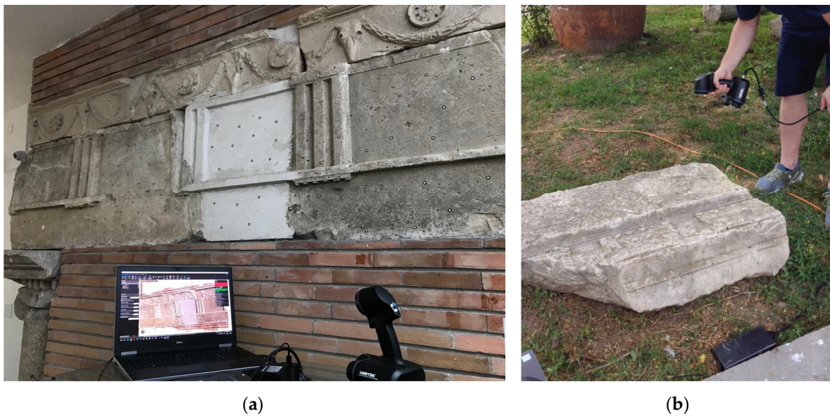
Figure 2. Snapshots captured during the 3D scanning process using structured light (a) indoor, (b) outdoor environments.
