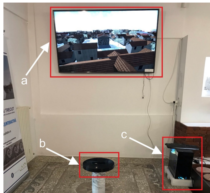
Figure 5. ISVS-B’s hardware architecture—highlighting visualization display (indicated with (a)), LeapMotion interaction sensor (indicated with (b)), and the process unit (indicated with (c)).
