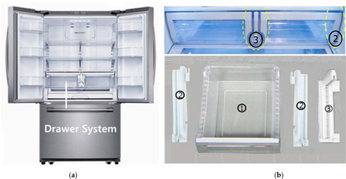
Figure 6. French-door refrigerator and drawer system. (a) French-door refrigerator; (b) mechanical components in a drawer: box ①, two guide rails ②, support center ③.
