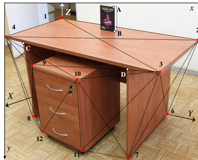
Figure 2. The right stereo picture with 3D precise linear network on the object (the points 1, . . . , 12 and A, B, C, D represent characteristic vertices of the object; X, Y, Z define a local 3D coordinate system; x, y represent pixel image coordinates).
