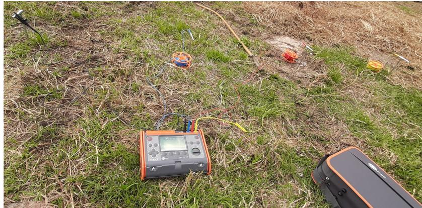
**Figure 5.** Measurement of the soil resistivity 1 (S1).
