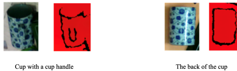
Figure 5. Objects with the same textures and different shapes, the left object is a cup with a handle and the right object is another side of the cup with the handle hidden. The depth image is next to the color image.
