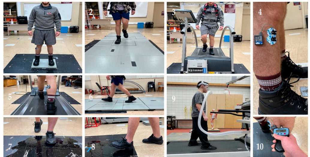
Figure 2. Biomechanics and physiology tests performed with occupational footwear. Various biomechanical and physiological human factors assessment in occupational footwear. (1) Static balance and postural stability, (2) Overground gait trials, (3) Treadmill gait trials, (4) Electromyography (EMG) from lower extremity muscles (tibialis anterior), (5) Treadmill workload used for fatigue induction with EMG (gastrocnemius pictured), (6) Overground dry surface gait trials, (7,8) Overground slippery surface gait trials, (9) Energy expenditure during treadmill workload, (10) Pressure pain threshold (PPT).
