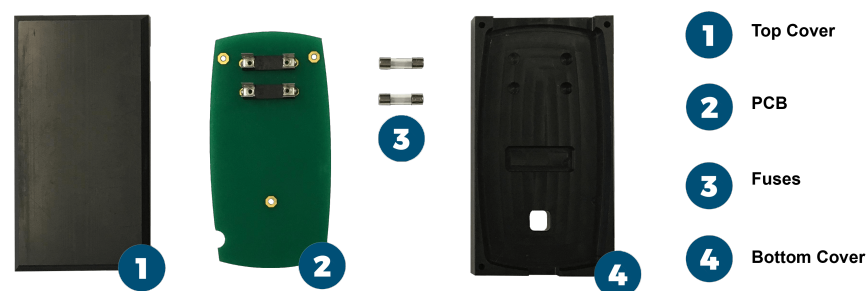
Figure 5. The parts of the mock-up mobile phone used for the learning and training scenarios.
