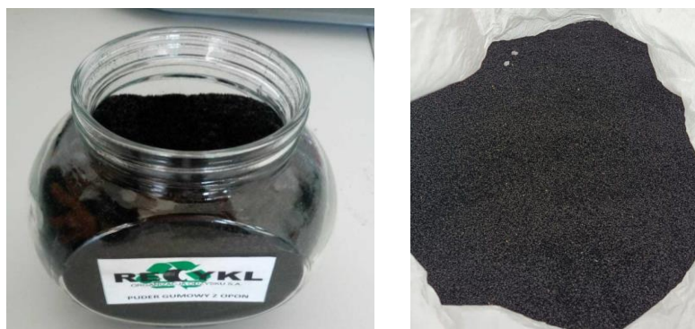
Figure 1. Rubber powder made from recycled tires. Source: Photo taken during the research.
