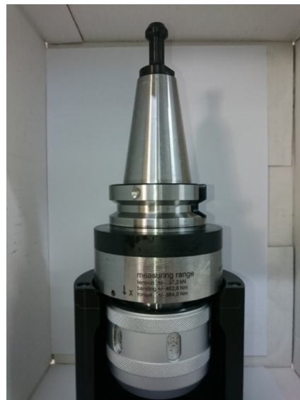
Figure 7. Tool holder embedded with sensors (Spike ® from Pro-micron GmbH).
