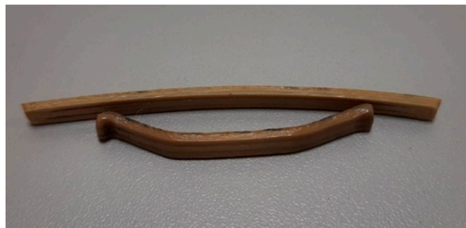
Figure 8. PEEK sample before and after DMA experiment.
