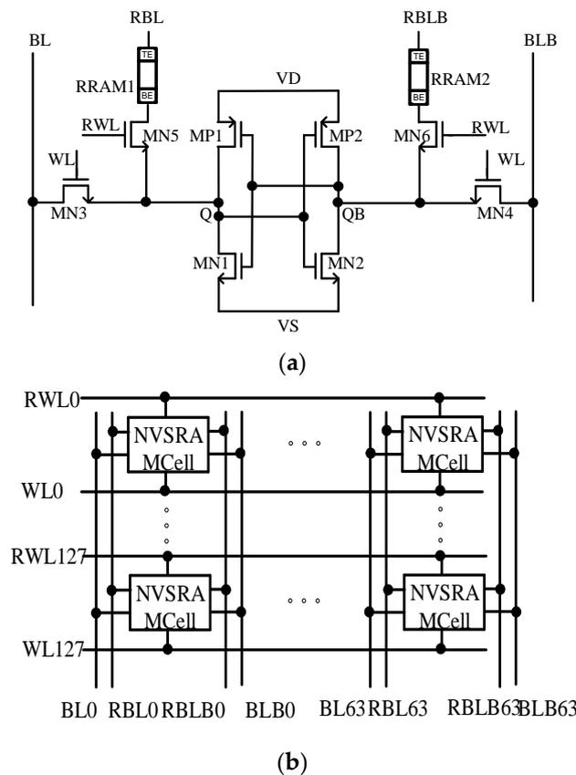
Figure 2. (a) 8T2R nvSRAM memory cell, (b) 128 × 64 array.
