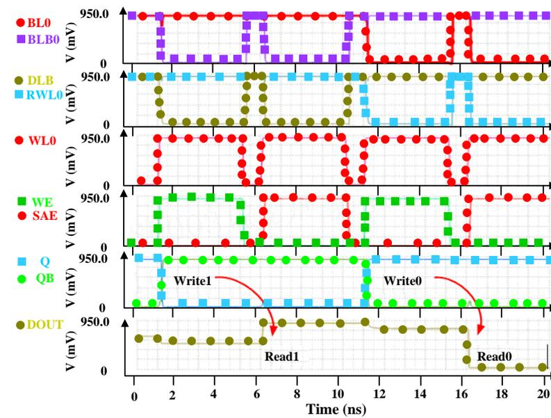
Figure 19. Simulation results for reading and writing speed.
