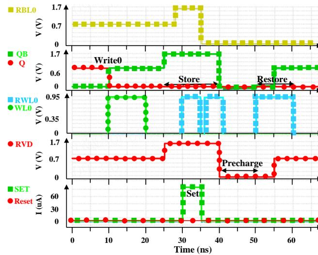
Figure 18. Simulation results for data storage and restoration circuit.
