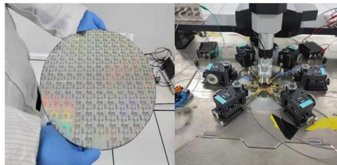
**Figure 12.** Die of nvSRAM and test environment.
