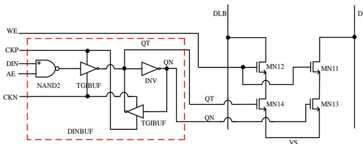
Figure 8. Write driver circuit.
