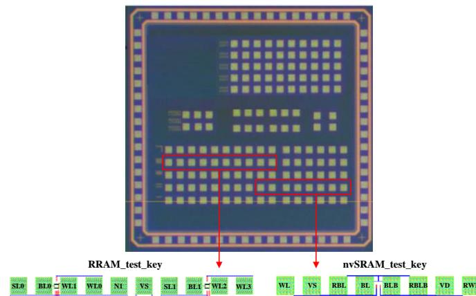
**Figure 11.** Micrograph of all test chip.
