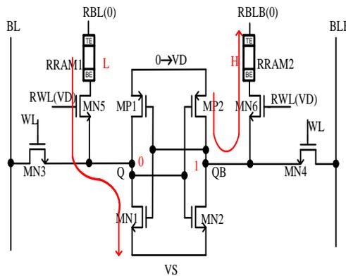
Figure 4. Data restoration operation.
