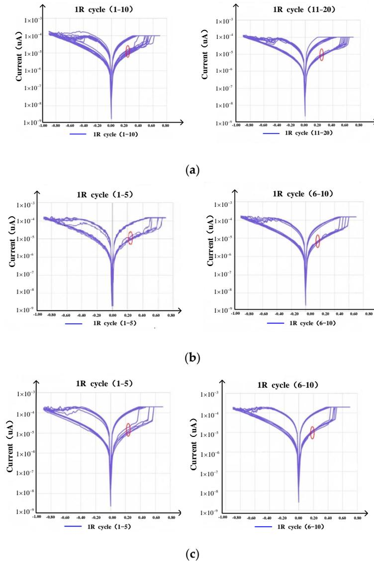
**Figure 13.** DC test results for 1T1R RRAM: (a) 20 cycles (current:100  $\mu\text{A}$ ); (b) 10 cycles (current: 150  $\mu\text{A}$ ); (c) 10 cycles (current: 200  $\mu\text{A}$ ).
