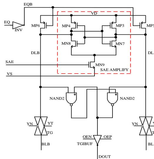
Figure 7. Read drive circuit.
