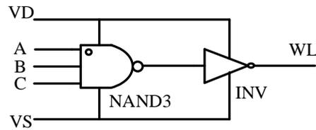
Figure 5. Row decoding circuit.
