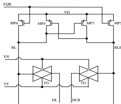
Figure 6. Column decoding circuit.
