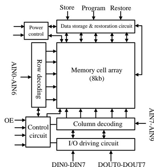
Figure 1. nvSRAM system structure.
