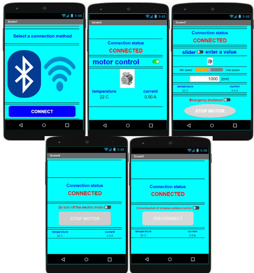
Figure 4. The interface of the developed mobile application with sequentially switched screens; from the left: screen 1, establishing a connection (Bluetooth or Wi-Fi); screen 2, enabling control; screen 3, motor rotational speed control (using a slider or entered value) with an emergency stop; screen 4, motor shutdown; screen 5, disconnection.
