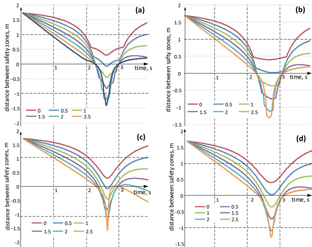
**Figure 8.** Distance in  $y$ -axis direction between safety zones for different lateral speeds (km/h) of the obstacle: (a) vehicle—rectangle, obstacle—circle; (b) vehicle—rectangle, obstacle—ellipse; (c) vehicle—ellipse, obstacle—circle; (d) vehicle—ellipse, obstacle—ellipse.
