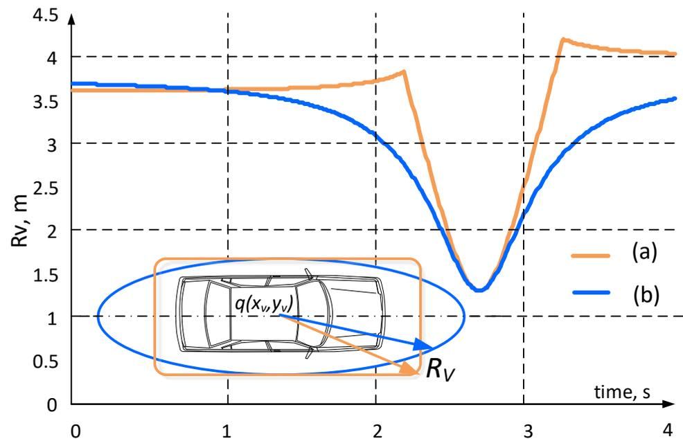
**Figure 6.**  $R_V$  parameter change depending on the shape of the safety zone around the vehicle: (a) rectangle, (b) ellipse.
