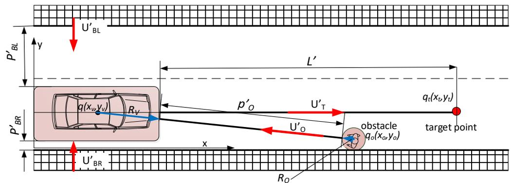
Figure 4. Introduction of vehicle and obstacle safety zones to the situation scheme.
