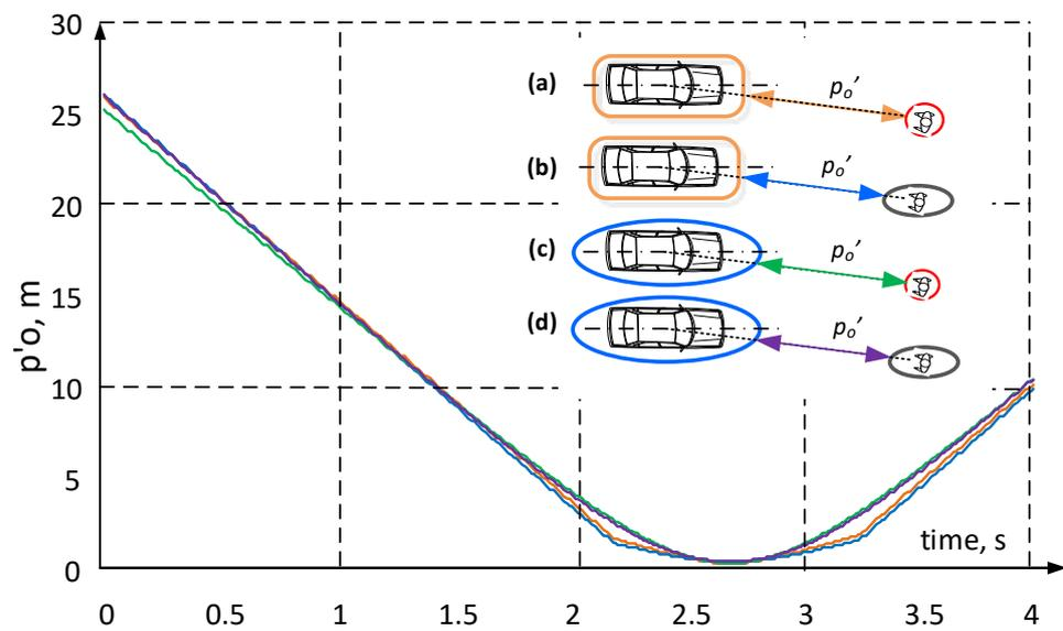
**Figure 7.** Change of  $p'o$  values, depending on the shape of the safety zone around the vehicle and the obstacle: (a) vehicle—rectangle, obstacle—circle; (b) vehicle—rectangle, obstacle—ellipse; (c) vehicle—ellipse, obstacle—circle; (d) vehicle—ellipse, obstacle—ellipse.
