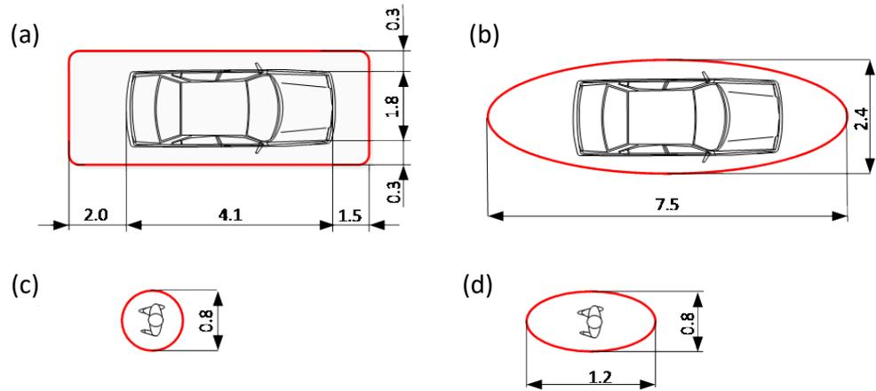
**Figure 5.** Size of the safety zone dimensions used in the simulation; (a) vehicle rectangular, (b) vehicle elliptical, (c) pedestrian circular, (d) pedestrian elliptical.
