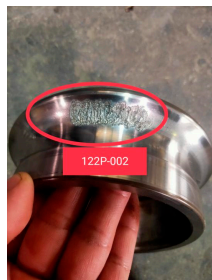
Figure 9. The actual faulty component of the engineering bearing.
