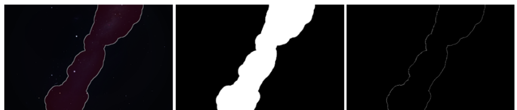
Figure 9. Left: RGB image. Middle: binary image. Right: edge image.
