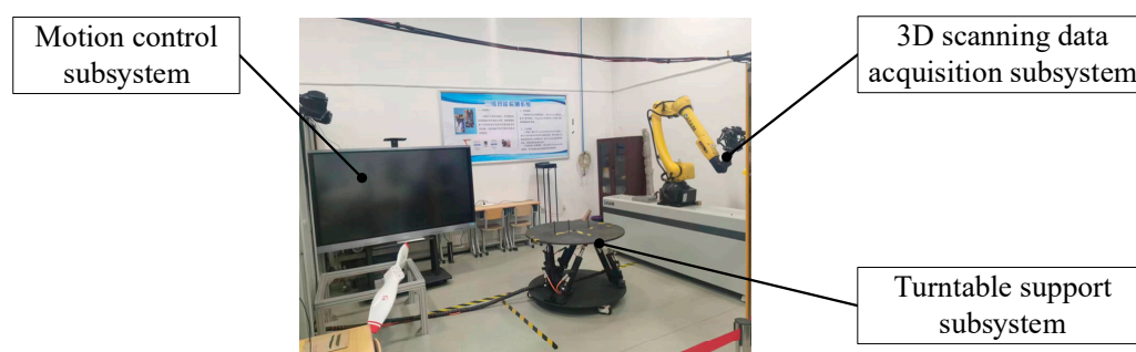
Figure 2. Automatic tracking type 3D scanning measurement system.
