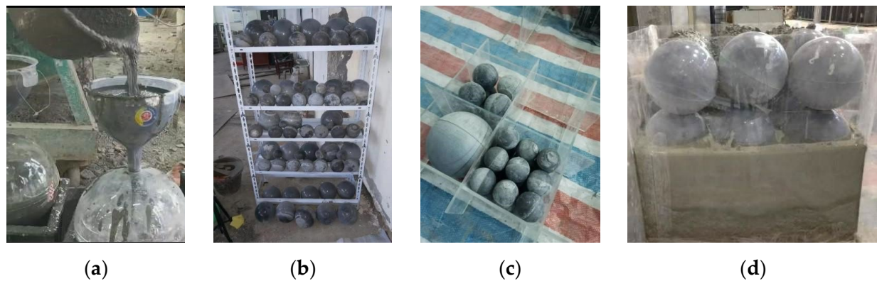
Figure 2. RFC specimen-making process. (a) Spherical aggregate is poured; (b) Aggregate demolding; (c) Aggregate accumulation; (d) SCC pouring.
