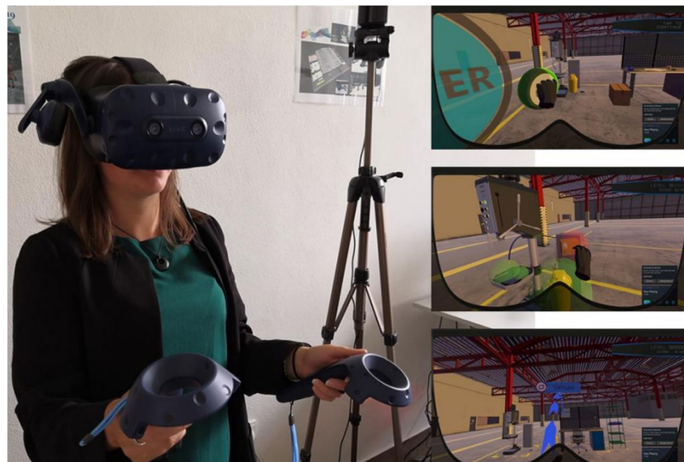
Figure 6. Application of gaming virtual reality based on Godot engine for teaching students at the University of Žilina (Reprinted from Ref. [36]).
