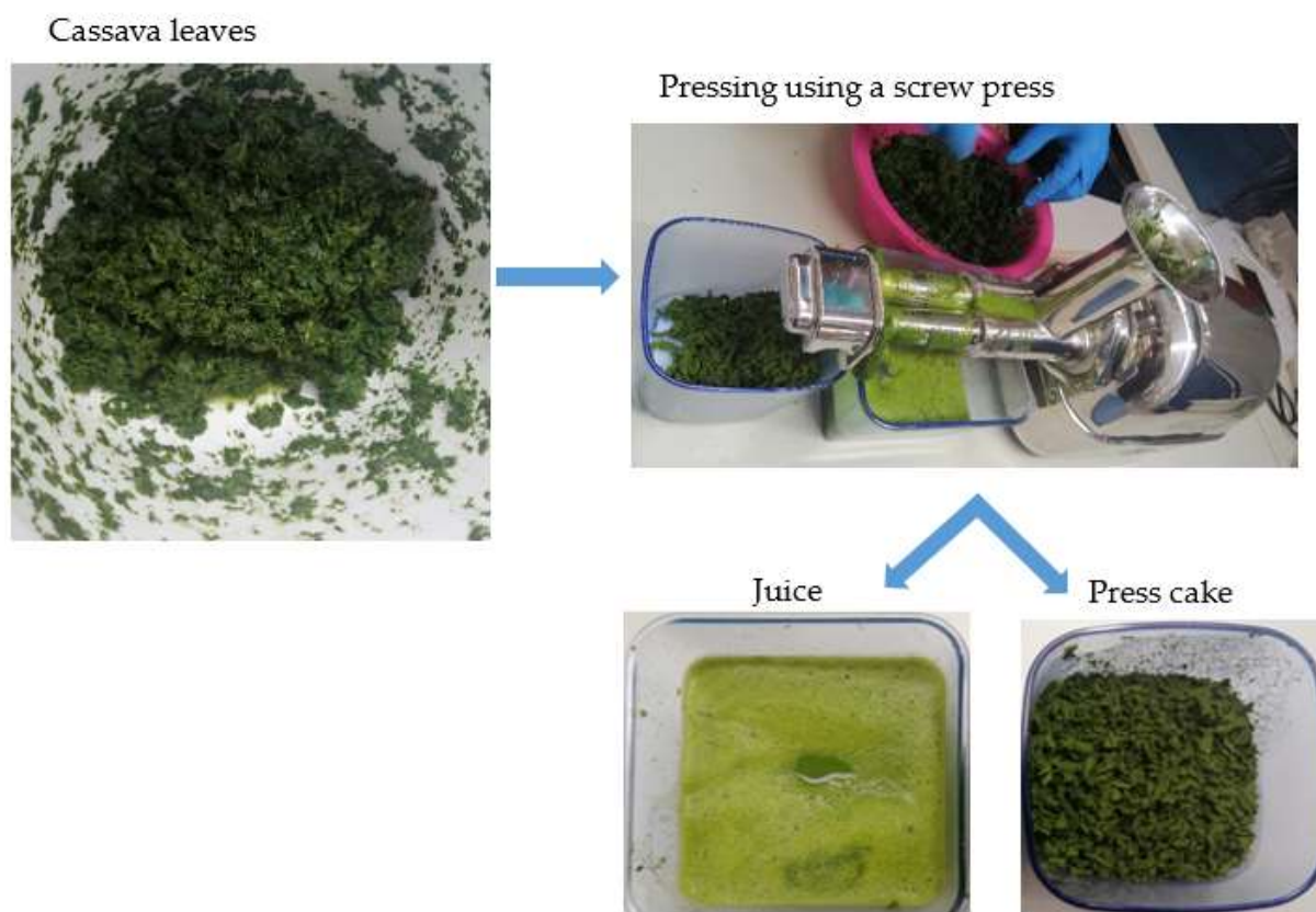
Figure 1. Screw pressing of cassava leaves into their fractions: juice, and press cake.
