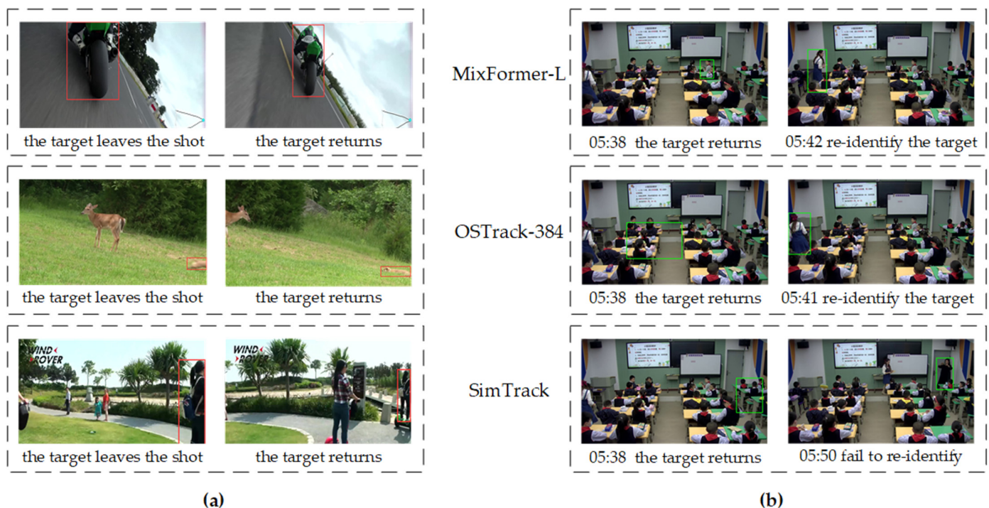
Figure 2. Factors of unsatisfactory tracking results. (a) Targets' frequently moving in and out of the shots. (b) The current SOT algorithms are generally weak in re-identification of the target after it leaves the shot.
