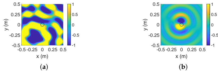
Figure 5. The true pressure field and recorded pressure field at 1500 Hz in the multiple sources scenario. The black circle denotes the receiver region. (a) the true pressure field; (b) the recorded pressure field.
