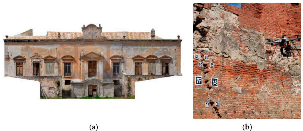
Figure 11. Orthophoto from close-range photogrammetry acquisition (a), from [155]; UAV image acquisition for marker-based structural defects monitoring (b), from [156].
