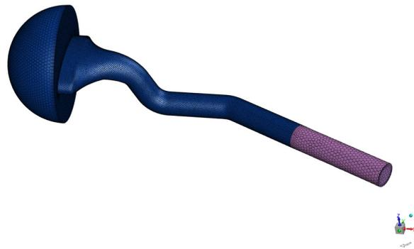
**Figure 3.** Mesh model of fluid domain of air intake dirty pipe.
