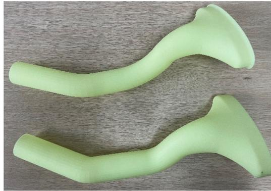
**Figure 18.** Simplified sample model of intake dirty pipe. The upper part is the sample after performance improvement, and the lower part is the sample before performance improvement.
