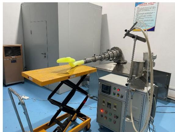
**Figure 19.** Flow resistance test device. The test piece is installed on a flow resistance device for testing.
