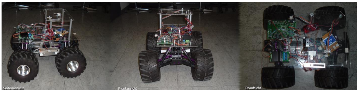
Figure 1. Attached robot on the Monster Truck HPI Savage 2.1.
