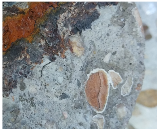
Figure 6. White halos around aggregates detected in the cores without microscopy needed.
